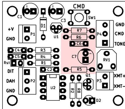
\***Note:** Resistor R5 was set to inject sidetone into an existing QRP transceiver. Other resistances may be required depending on your radio's sidetone requirements. Jumpering R5 (shorting) will allow a Piezo buzzer or small speaker to be used.
