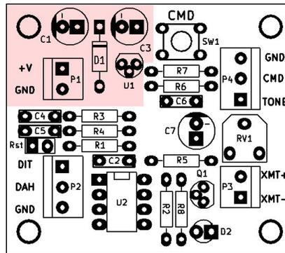
2. ( ) Power Supply Testing. Connect a 4-15V power source to P1 observing power polarity. Screws on P1 are shipped in the fully closed position. Using a DMM measure U2 pin 8 to ground. One of the mounting holes can be used as ground as well as any GND pin. There should be approximately 3.3V at this point. Disconnect power from P1.
